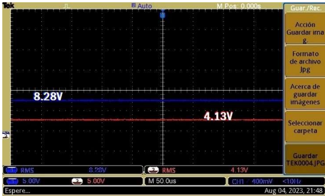
Figure 17 Reducer mode with low V_{in} seen in oscilloscope
