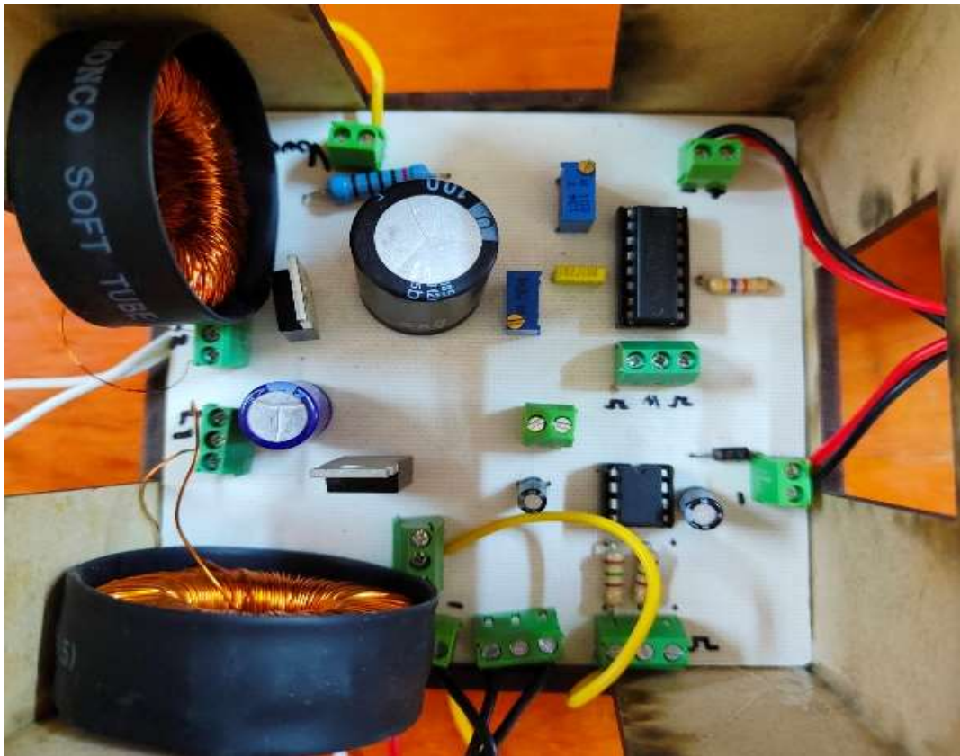
Figure 15 PWM control circuit and SEPIC converter
